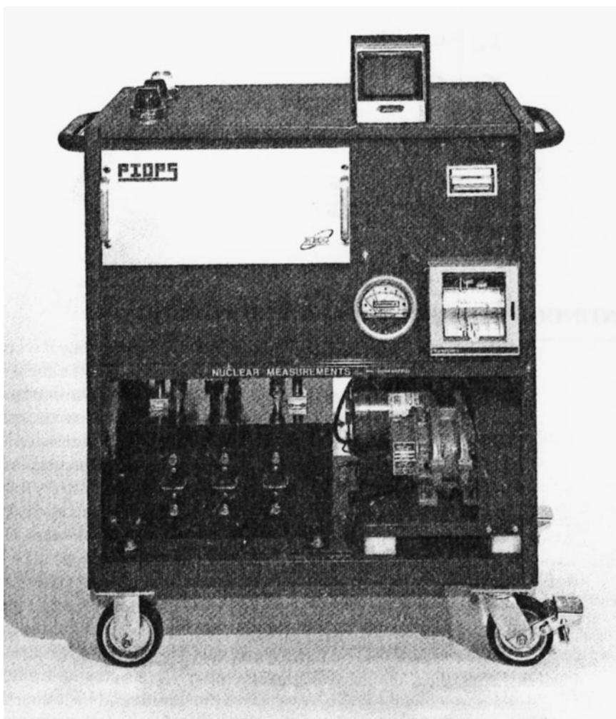
Figure 13-13. Continuous aerosol monitor for simultaneously measuring alpha, beta, and gamma activity at a sampling rate of 1 cfm (28.3 Lpm). The sensitivity at this sampling rate is 10^{-12} \mu\text{Ci/mL} ( 0.037 \text{ Bq/m}^3 ) of beta-gamma and of alpha activity. (Courtesy of Nuclear Measurements Corp.)
