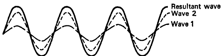
Figure 2-12. The addition of two waves of equal frequency and in phase.
